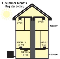
During warm outside temperatures, OPEN registers on upper floor and PARTIALLY CLOSE registers on first floor &/or basement.
