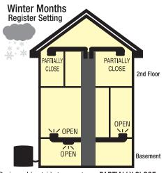
During cold outside temperatures, PARTIALLY CLOSE registers on upper floor and OPEN registers on first floor &/or basement.
